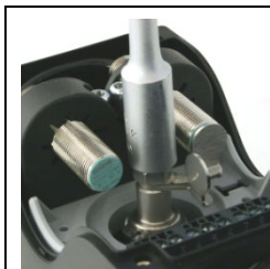
Fig. 3: Loosen nut screw
