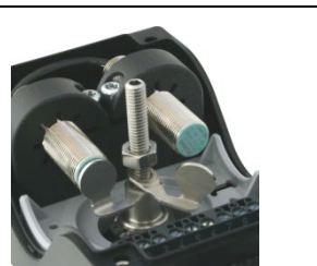
Fig. 5: Fixation of cam 2
